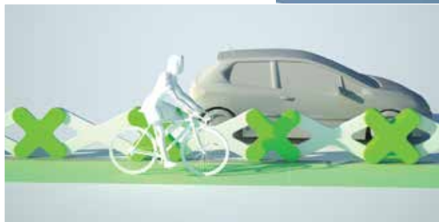
TOP Fast Lanes is a portable, modular, flat-pack system for establishing bike lanes.
